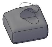
You can convert a surface or solid to a NURBS surface with the Convert to NURBS tool. Use Show CV to display the vertices for editing with the gizmo along with the other tools on the Control Vertices panel.
