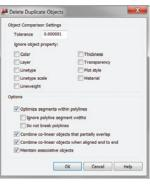
Control OVERKILL settings in the dialog box. Specify which object properties to ignore along with whether or not to optimize polyline segments and/or combine co-linear objects. The tolerance value controls the precision by which OVERKILL will operate.
